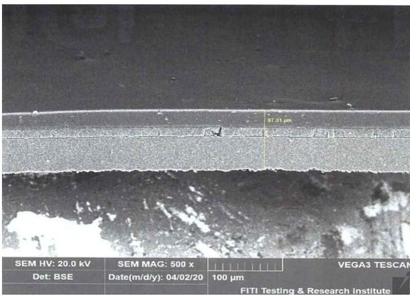
[Fig. Thickness of Anti-migration Film]
