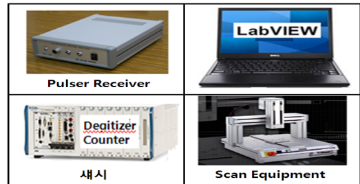
[Fig. 1] The composition of auto image inspection system
