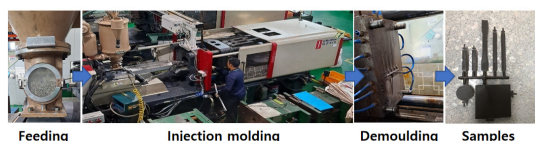
Fig. 2. Schematic diagram of injection molding
