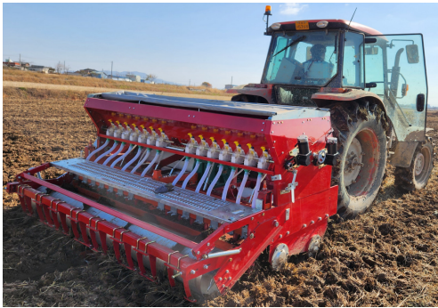
Fig. 2. Fertilizing and sowing device attached with tractor.
