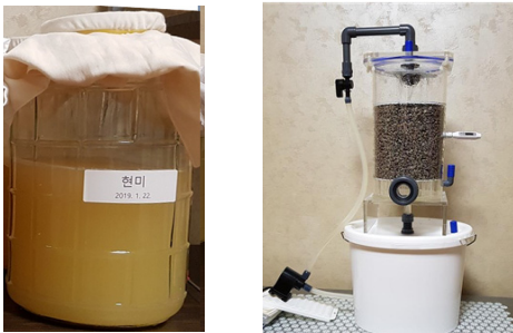
Fig 1. Surface fermentation (left) and fixed fermenter (right)
