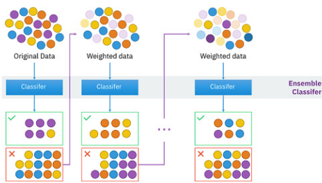
Fig. 2. The concept of boosting for the construction of the SAMME model
