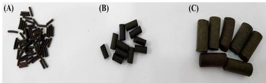
Fig. 3. Propellant shape of XXmm high explosive propellant single-perforated cylinder type(A), small size multi-perforated cylinder type(B) and large size multi-perforated cylinder type(C)
