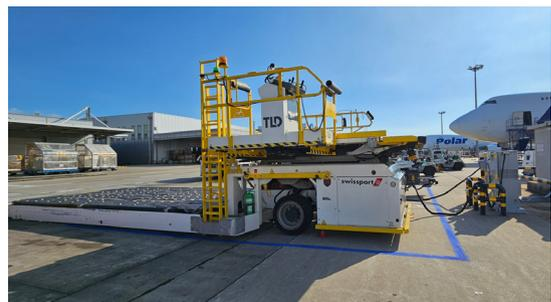
Fig. 6. Electric Powered Upper-deck Loader at ICN
