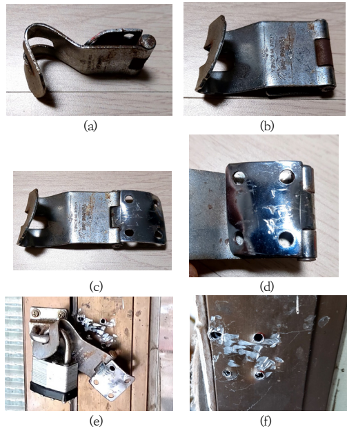
Fig. 4. Actual case of door lock hasp failure (a) Door lock hasp failure top view (-z direction) (b) Door lock hasp failure front view (+y direction) (c) Door lock hasp failure with screw mounting surface (d) Screw mounting surface of door lock hasp failure (e) Door lock hasp failure with lock (f) Entrance door surface where hasp installed
