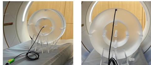
Fig. 1. Measurements of dose change according to kVp
