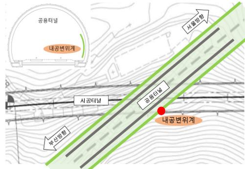
Fig. 6. Installation of convergence gauges in the structure of the operating tunnel
