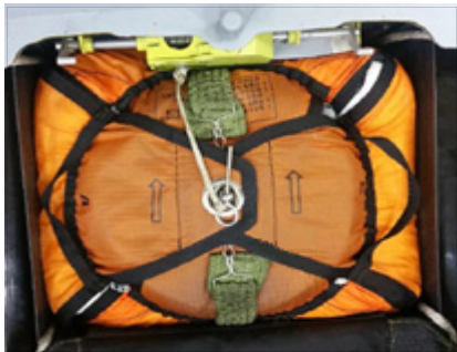
Fig. 4. The installed parachute
