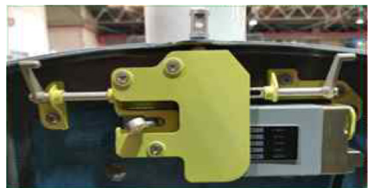
Fig. 6. Parachute door locking mechanism configuration
