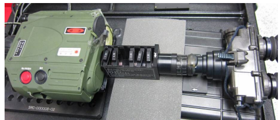
Fig. 6. 3rd generation night vision goggle black spot occur test
