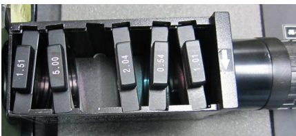
Fig. 4. Light attenuation filter for 1.54 \mu m laser
