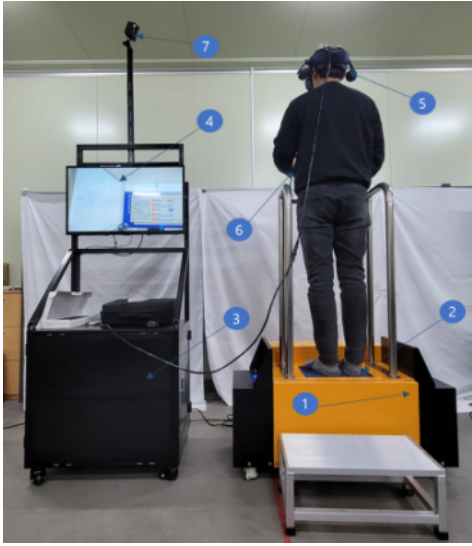
Fig. 4. Virtual Reality-Based Blasting Vibration Simulator
