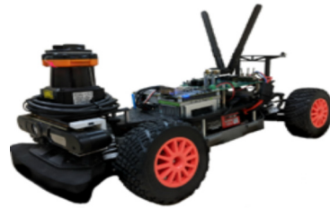
Fig. 2. Hardware platform of F1TENTH[9]
