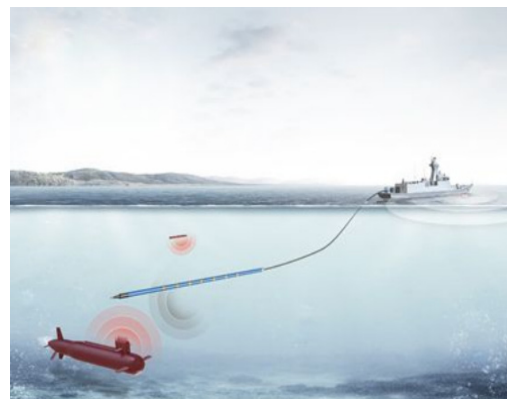
Fig. 1. Towed Array Sonar System for Export[10]
