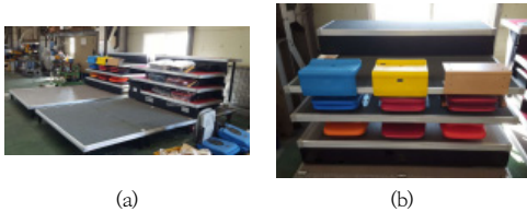
Fig. 6. Photographs of small testbeds for measuring stress change data of the grandstand structure
