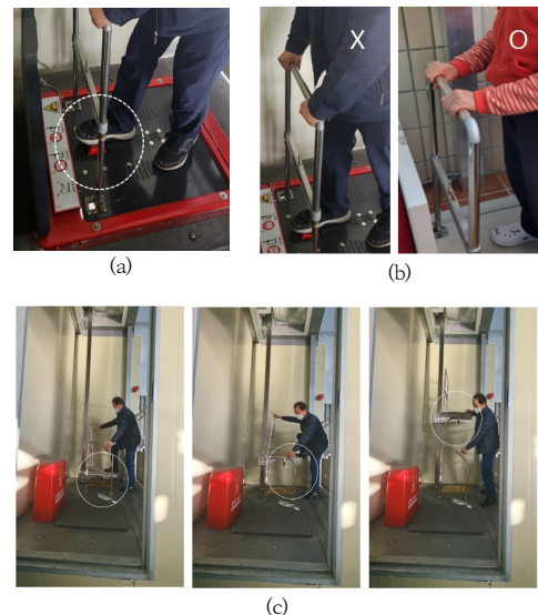
Fig. 3. Example of an accident when using an elevating evacuator (a) Press pedal (b) Safety handle (c) Lift plate
