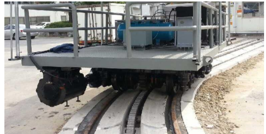
Fig. 5. Carbody running on the test track
