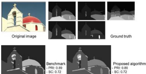
Fig. 18. Comparison of image segmentation(1)
