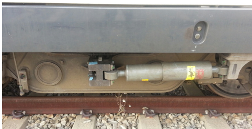
Fig. 3. Yaw damper installation change
