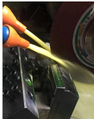
Fig. 3. Cutting process of quenched ball stud
