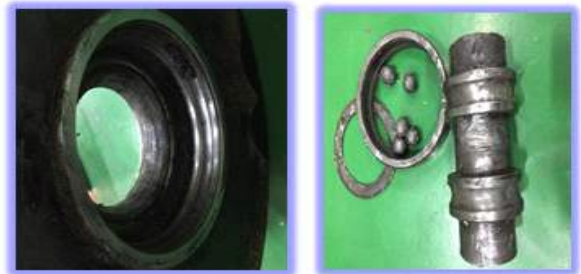
(c) Wheel bearing damage
